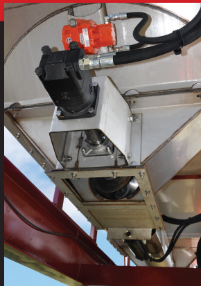
Hydraulic Operated Clean Out Doors
